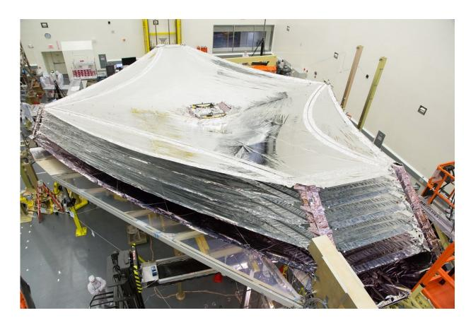
The sunshield of NASA's James Webb Space Telescope will prevent the background heat from the sun from interfering with the telescope's infrared sensors. It was designed by Northrop Grumman Aerospace Systems in Redondo Beach, California. Credit: Northrop Grumman
