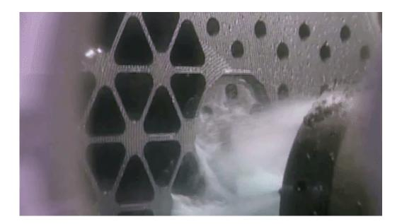
Because the weight of a payload is so critical to cost-effectively launch it into space, each one of Webb telescope's primary mirror segments was "light-weighted." The process involved cutting away most of the backside of each mirror segment while leaving structural ribs for support, thus reducing the weight while maintaining the strength and integrity of the mirror. Credit: NASA
