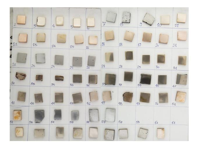
64 metal samples of using variable copper-tin-arsenic compositions created to use in the study. Credit: M. Radivojevic
