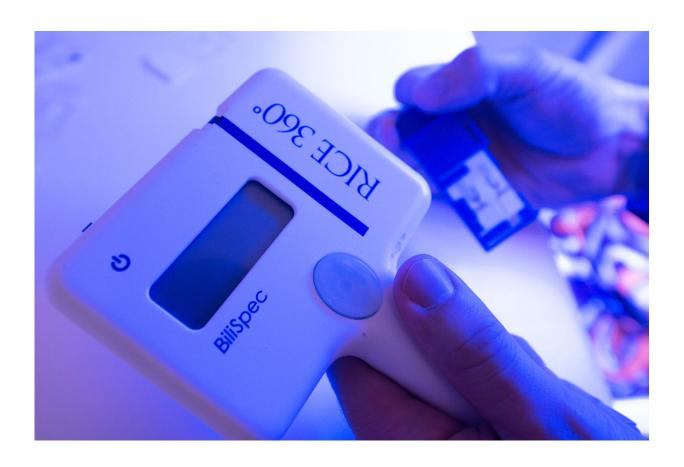
BiliSpec is a low-cost, battery-powered reader designed to diagnose jaundice by immediately quantifying serum bilirubin levels from a small drop of whole blood. Credit: Jeff Fitlow/Rice University
