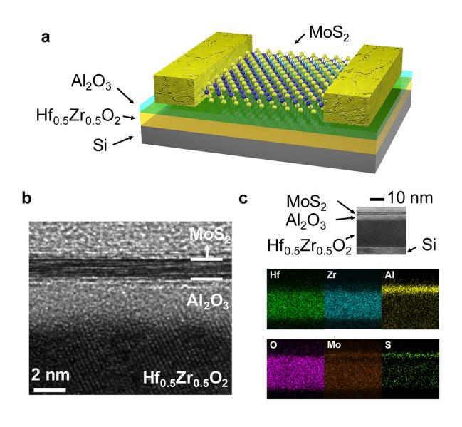
A new type of transistor (a) harnesses a property called negative capacitance. The device structure is shown with a transmission electron microscopy image (b)
