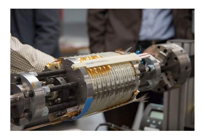
The Florida State University-headquartered National High Magnetic Field Laboratory has shattered another world record with the testing of a 32-tesla magnet — 33 percent stronger than the world's strongest superconducting magnet used for research and more than 3,000 times stronger than a small refrigerator magnet. Credit: National MagLab
