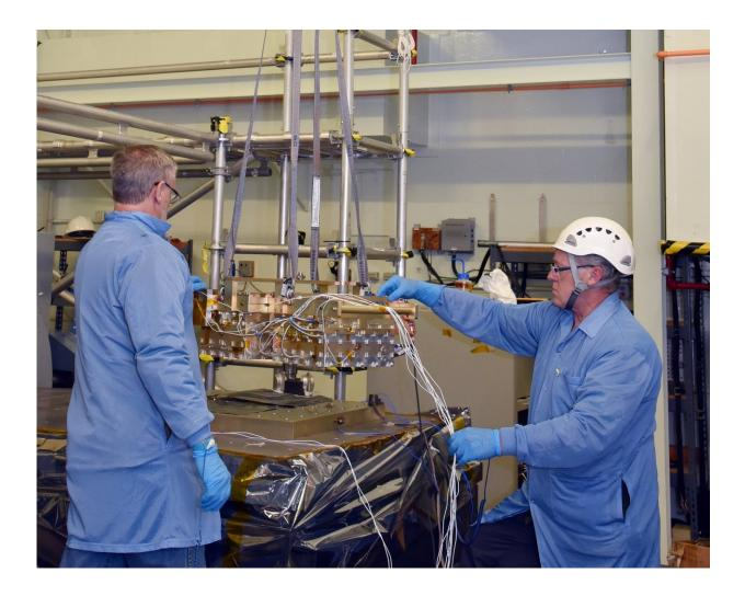
LCRD engineers prepare Flight Modem 2 for vibration testing. Credit: NASA Goddard/Barbara Lambert
