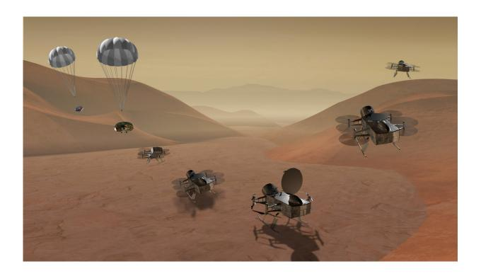
Dragonfly is a dual-quadcopter lander that would take advantage of the environment on Titan to fly to multiple locations, some hundreds of miles apart, to sample materials and determine surface composition to investigate Titan's organic chemistry and habitability, monitor atmospheric and surface conditions,
