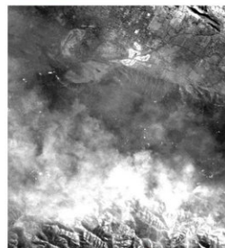
1000 nm channel: sees smoke
