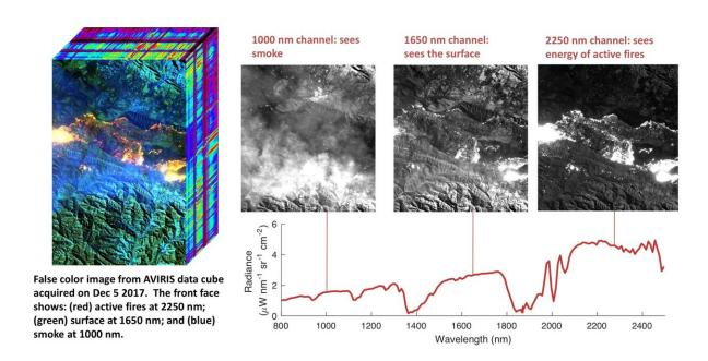
NASA's Airborne Visible Infrared Imaging Spectrometer, aboard a NASA Armstrong Flight Research Center high-altitude ER-2 aircraft, flew over the Southern California wildfires on Dec. 5, 2017 and acquired this false-color image. Active fires are red, ground surfaces are green and smoke is blue. Credit: NASA/JPL-Caltech
