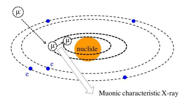
Concept of Muonic Characteristic X-ray. Credit: Osaka University
