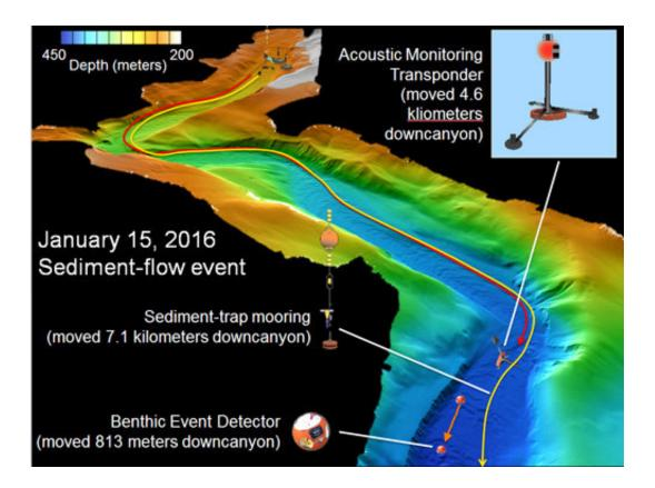
This illustration shows some of the instruments that were moved downcanyon by a sediment-flow event on January 15, 2016. Surprisingly, some large, heavy instruments traveled farther than did smaller, lighter instruments. Credit: 2017 MBARI
