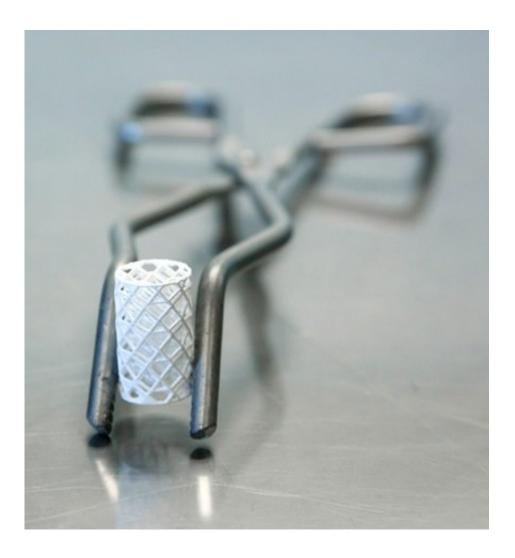
The geometric ceramic structure of the test catalytic converter designed on the computer. Specialists at Empa coated it with the catalytically active layer and tested the cleaning effect in an artificial stream of exhaust gas. Credit: Swiss Federal Laboratories for Materials Science and Technology
