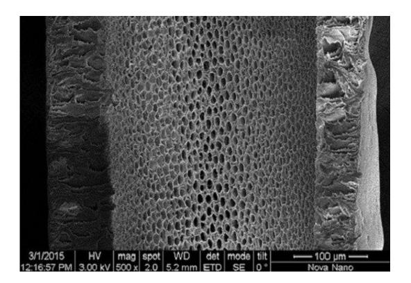
A superior membrane, with a higher pore density, is produced through synthesizing this polyacrylonitrile nanofiltration membrane using an ionic liquid solvent. Credit: © 2017 Susana Nunes
