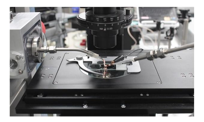
High resolution atmospheric pressure mass spectrometry imaging system. Credit: Daegu Gyeongbuk Institute of Science and Technology (DGIST)
