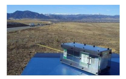
Researchers test the CubeSat, which is communicating with a ground station about four miles away. Credit: University of Colorado Boulder
