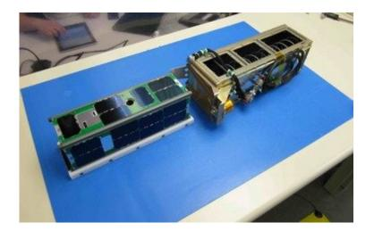
The CubeSat just before it was brought into the launch facility. Credit: University of Colorado Boulder
