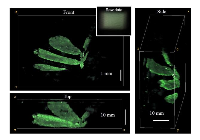
The researchers used the DiffuserCam to reconstruct the 3-D structure of leaves from a small plant. They plan to use the new camera to watch neurons fire in living mice without using a microscope. Credit: Laura Waller, University of California, Berkeley
