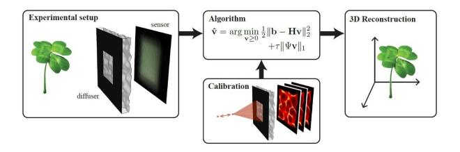
The lensless DiffuserCam consists of a diffuser placed in front of a sensor (bumpson the diffuser are exaggerated for illustration). The system turns a 3-D scene into a 2-D image on the sensor. After a one-time calibration, an algorithm is used to reconstruct 3-D images computationally. The result is a 3-D image reconstructed from a single 2-D measurement. Credit: Laura Waller, University of California, Berkeley
