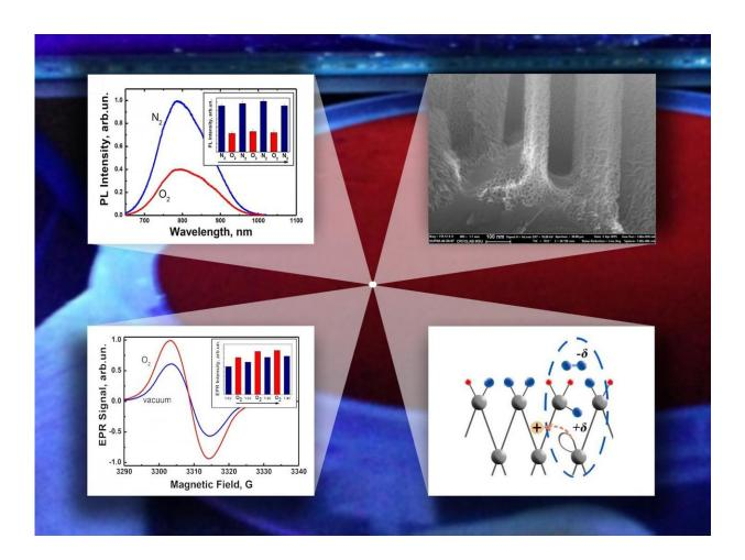
Principle of the operation of the sensor based on porous silicon nanowire arrays. Credit: Liubov Osminkina
