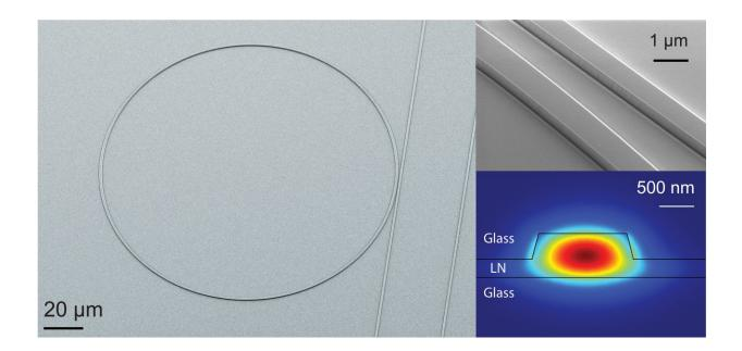
SEAS researchers have designed a micro-ring and micro-racetrack resonators made from lithium niobate, a material previously thought unworkable for highquality, small scale optical devices Credit: Loncar Lab/Harvard SEAS
