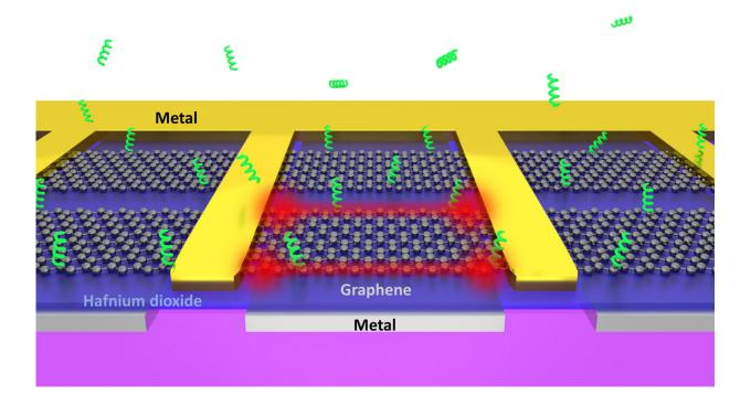
Atomically sharp edges of electrically driven graphene can act as 'tweezers' that rapidly trap biomolecules from the surrounding solution. Credit: In-Ho Lee, University of Minnesota
