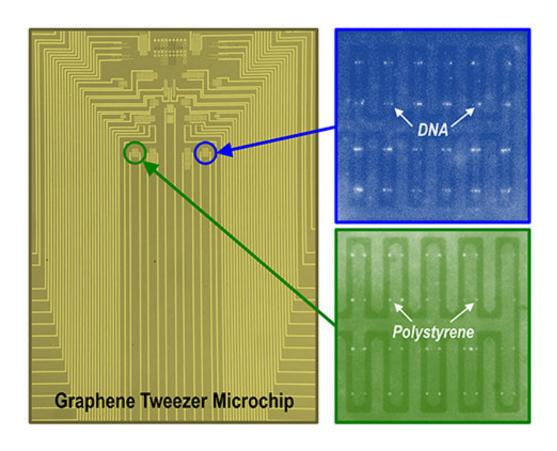
The University of Minnesota team produced a microchip containing a large array of graphene electronic tweezers. Fluorescence images show DNA molecules and polystyrene nanoparticles trapped on the chip. Credit: Barik et al., University of Minnesota
