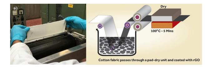
Demonstration of laboratory-scale pad-dry unit and illustration of the pad-dry unit process. Illustration by Daniel Wand. Credit: Karim et al. ©2017 American Chemical Society
