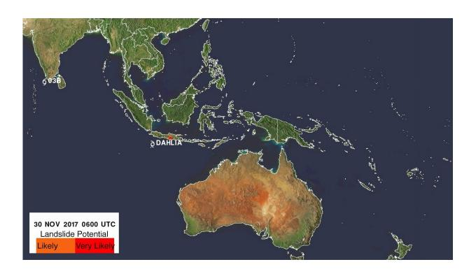
This landslide potential map was created based on rainfall estimates from near real-time Multi-satellite Precipitation Analysis (TMPA) data. The map shows that heavy rainfall during the past week resulted in an area of potential landslides on the slopes of southern Java. Credit: NASA/JAXA, Hal Pierce
