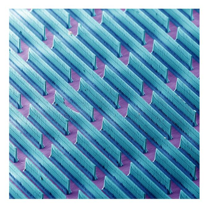
Microscopic image showing the walls formed to mimic the adhesion characteristics of gecko feet. Credit: Georgia Tech
