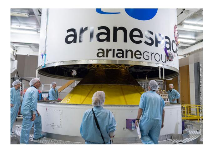
Four Galileo satellites being encapsulated by the protective payload fairing on 7 December, completing the Ariane 5 for flight VA240, scheduled for 12 December 2017. Credit: ESA-CNES-Arianespace / Optique video du CSG – JM Guillon
