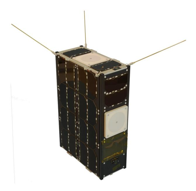
ESA's GomX-4B CubeSat will test intersatellite links and propulsive orbit control for future constellation operations, working with twin GomX-4A, which is owned by the Danish Ministry of Defence. Credit: ESA/GomSpace
