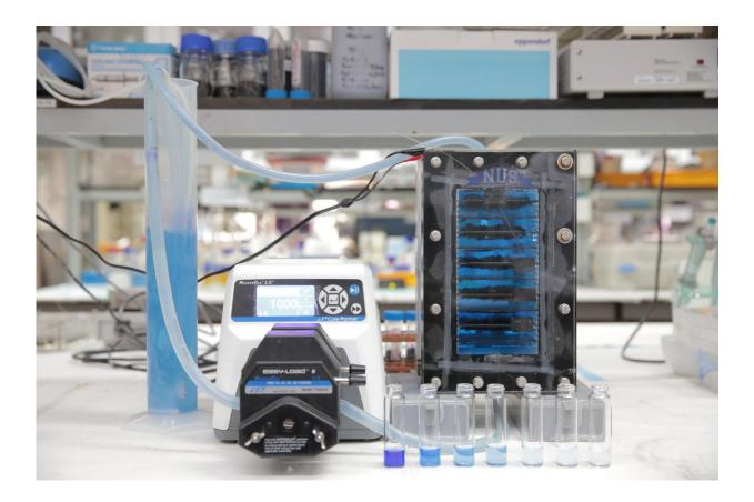
NUS scientists created a robust, highly efficient and easy to operate water purification system for industrial wastewater. This NUS invention operates on low electrical power and does not generate secondary waste, such as sludge, that requires further costly residual waste processing such as incineration. Credit: National University of Singapore
