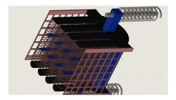
A schematic for a prototype of the proposed water cloaking device. It consists of wires and coils that create an electromagnetic field that acts on dissolved ions to move water around the object. Credit: Duke University
