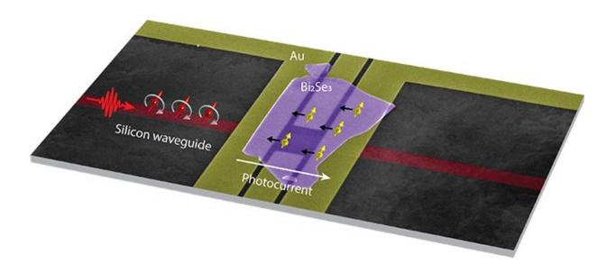
False-colored electron microscope image of the University of Minnesota device. The blue area marks the topological insulator on top of the optical waveguide in red. Credit: University of Minnesota
