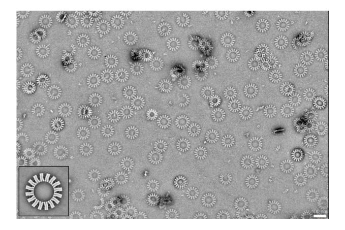
DNA-origami "gear-wheels" self-assembled from V-shaped building blocks. Image taken with a Titan Krios G2 300 kV cryo-elektron microscope. Scale-bar: 100 nm. Credit: Hendrik Dietz / TUM
