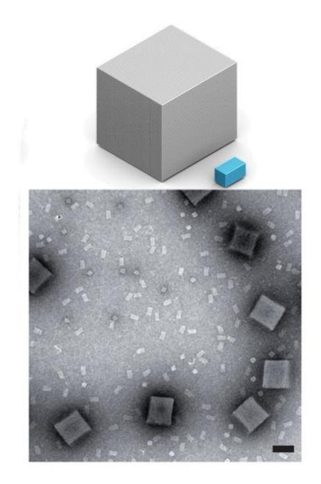
The top model and the bottom TEM image shows how the size of a 536 megadalton DNA brick cuboid (grey) compares to that of a much smaller 4.3 megadalton origami cuboid (light blue). Credit: Wyss Institute at Harvard University
