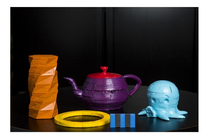
The UW team also demonstrated how to use the magnetic properties of some 3-D printed material to invisibly encode static data in the objects above, which could be useful for inventory tracking or to help robots interact with them. Credit: Mark Stone/University of Washington
