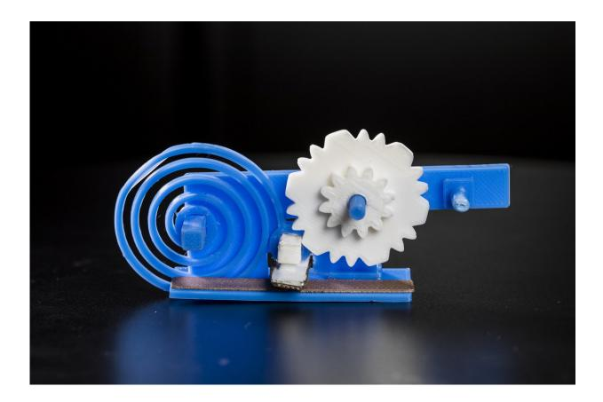
The 3-D printed gears (in white) and spring (blue spiral) toggle a switch (white box with grey surface) made of conductive plastic. The switch changes the reflective state of a 3-D printed antenna (gray strip) to convey useful data to a WiFi receiver. The shape of the gears and the speed at which they move encode the digital data. Credit: Mark Stone/University of Washington
