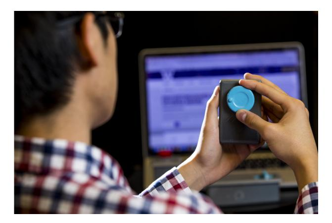
The UW team of computer scientists and electrical engineers also 3-D printed plastic scroll wheels, sliders and buttons that can wirelessly interact with computers, phones and other WiFi-connected devices. Credit: Mark Stone/University of Washington
