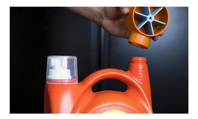
UW engineers have developed the first 3-D printed plastic objects that can connect to other devices via WiFi without using any electronics. The 3-D printed attachment above can sense how much laundry soap is being used -- and automatically order more when the bottle is running low. Credit: Mark Stone/University of Washington
