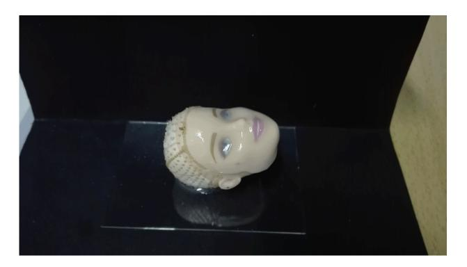
Bacterial cellulose producing bacteria are printed onto a non-planar surface (silicone face) to create personalized cellulose scaffolds. Credit: Manuel Schaffner and Patrick A. Rühs
