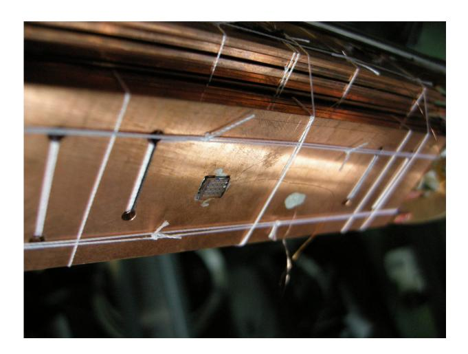
A chip with a Coulomb blockade thermometer on it is prepared for experiments at extremely low temperatures. Credit: University of Basel, Department of Physics
