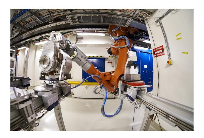
As in the ISOLDE facility, the targets at MEDICIS have to be handled by robots because they are radioactive. Credit: Maximilien Brice/CERN
