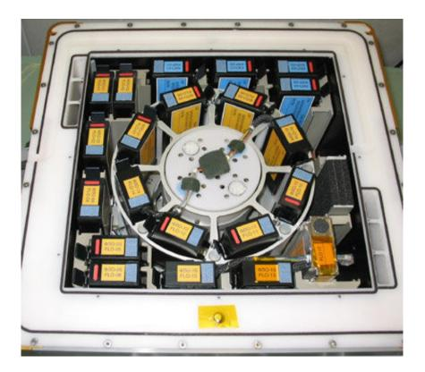
Kubik is a 37x 37cm temperature-controlled incubator for studying biological samples. Two Kubik are currently on the International Space Station, housed in the Columbus module. The hardware is loaded with biological samples housed in Experiment Units. Kubik can be automatically operated for a preset timeline or manually operated by astronauts. Credit: ESA
