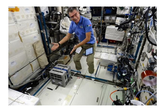
ESA astronaut Paolo Nespoli prepares the Kubik hardware. Kubik is a controlledtemperature incubator for studying biological samples. After preparing the unit, Paolo loaded it with the muscle, retinal, and stem cells being studied by Italian researchers in an experiment coordinated and funded by Italy's ASI space agency. Credit: ESA/NASA
