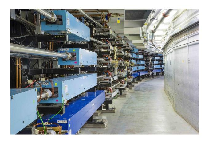
Magnets that steer and focus the electron beams in Jefferson Lab's Continuous Electron Beam Accelerator Facility. Credit: DOE's Jefferson Lab
