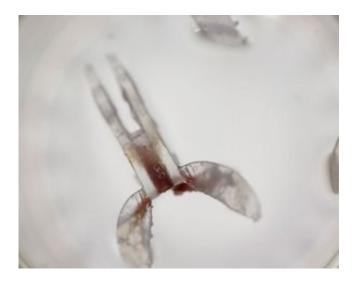
Biorobots made from sea-slug muscle tissue attached to a 3-D-printed frame. Credit: Case Western Reserve University
