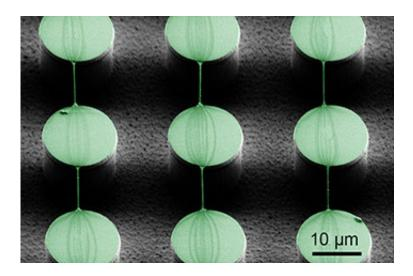
To create nanowires the researchers placed a droplet on the surface, and then dragged the droplet laterally, leaving strands of the material spanning the pillars. Credit: KTH Royal Institute of Technology
