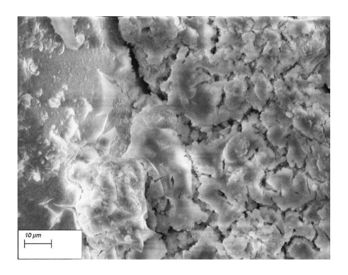
The material works by absorbing water that exists within the concrete to form crystals . Credit: Brunel University
