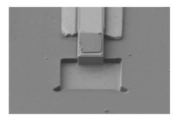
An etched facet semiconductor laser with an air gap reflector. Credit: Optical Society of America
