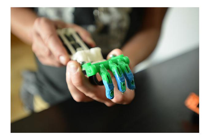
A low-cost 3-D printed prosthetic hand. Credit: M.R.Nuckels via Wikimedia
