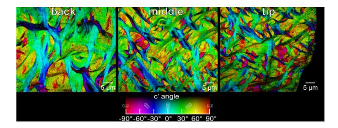
An X-ray-based technique known as PIC mapping shows the size and orientation
