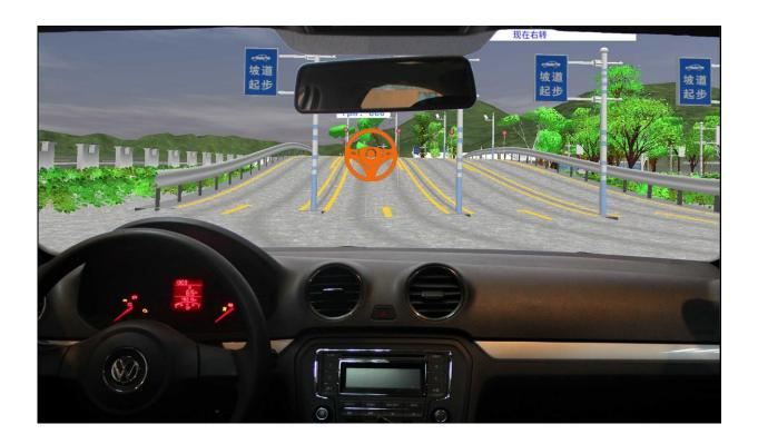
A real car has been turned into a driving simulator. The virtual environment is visible in front of the window. Credit: KIT, IMI
