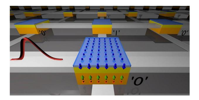
In this schematic of a magnetic memory array, an ultrafast electrical pulse switches a magnetic memory bit. Credit: Jon Gorchon
