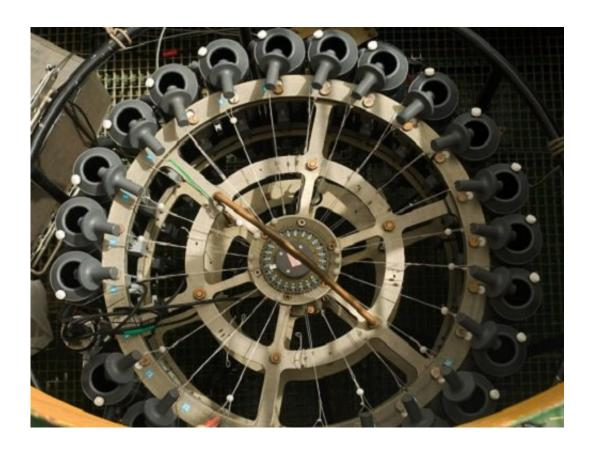
At specific depths, bottles of the CTD rosette are closed and water is collected for the analysis of microbial communities and potential explanatory variables (e.g. nutrient concentrations). Credit: KAUST
