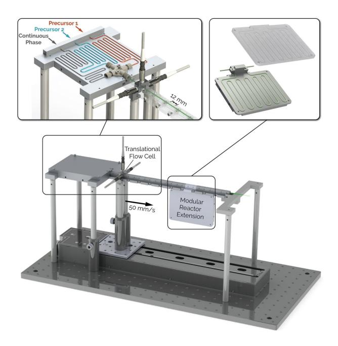
The exploded view of NanoRobo, highlighting the heating and reactor extension modules. Credit: North Carolina State University
