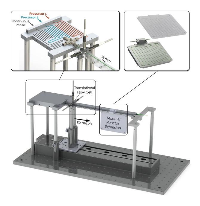
The exploded view of NanoRobo, highlighting the heating and reactor extension modules. Credit: North Carolina State University
