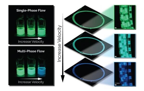
Effect of controlling mixing time by changing flow velocity on the emission wavelength (i.e., fluorescence color) of the resulting perovskite quantum dots. Credit: North Carolina State University
