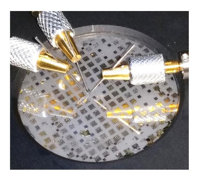
Image shows wafer-scale processed AlGaN/GaN sensors being tested. Credit: Georgia Tech Lorraine
