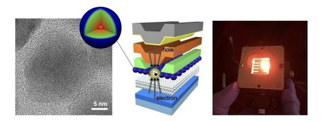
A collage showing contains a transmission electron microscopy image of the improved quantum dot and its representation (left), the schematic of the device which nicely illustrates 'current-focusing' idea (middle), and the device under operation (right). Credit: LANL
