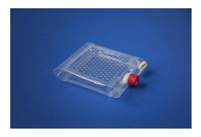
The mini laboratory is 150 mm long, 120 mm wide and 20 mm high. The screw cap is made using 3D printing. Hydrophilic spots are visible on the upper interior surface of the bag. Credit: Fraunhofer-Gesellschaft
