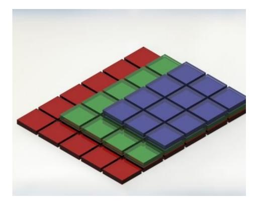
Stack instead of mosaic: the perovskite layers each absorb only part of the light spectrum. Credit: Empa
