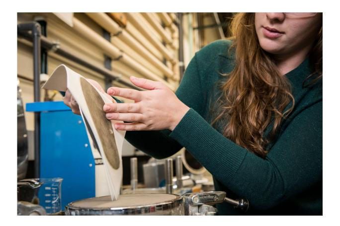
The finished sheet of "smart" paper is pulled off the press. Credit: Mark Stone/University of Washington
