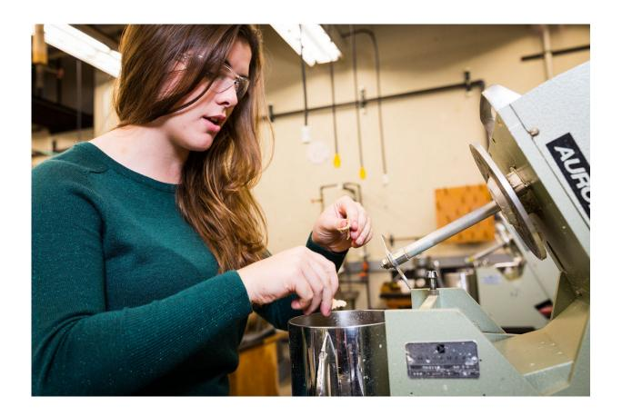
The process begins with dried sheets of softwood pulp. Here, undergraduate student Demi Lidorikiotis tears the dry pulp into small pieces at the start of the papermaking process. Credit: Mark Stone/University of Washington
