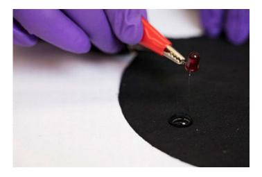
A water droplet disrupts the electrical connection in the paper, causing the light to turn off. Credit: Mark Stone/University of Washington
