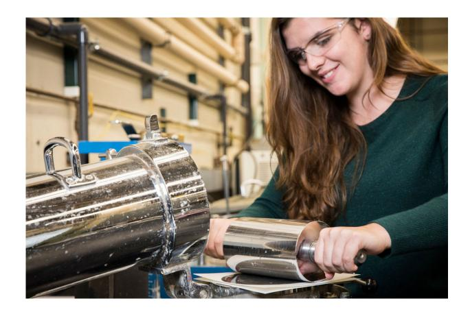
Demi Lidorikiotis uses a roller to manually press out any remaining water. Credit: Mark Stone/University of Washington
