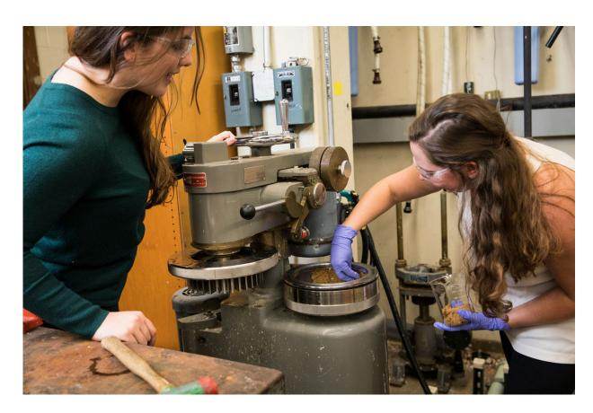
Next, the pulp slurry is placed in a different machine that splits the wood fibers, allowing chemicals added later to better bind to the pulp. Undergraduate students Demi Lidorikiotis, left, and Sydney Fry tend the mixture. Credit: Mark Stone/University of Washington
