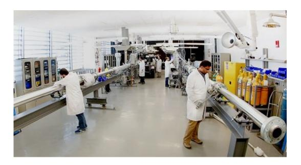
Students test fuel ignition chemistry using two shock tubes at the KAUST Clean Combustion Research Center. Credit: KAUST
